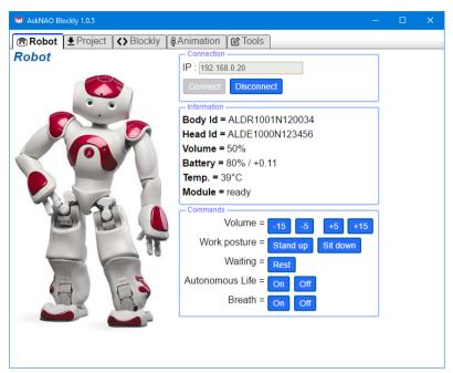
**Body Id** and **Head Id** are the serial numbers of the robot (respectively the number of the body and head).
